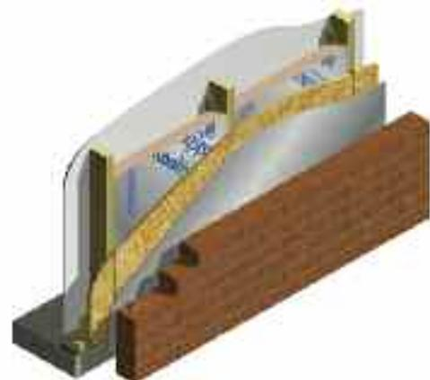
Wall 2 - Mineral Fibre and Studs Replaced with 75 mm of Rigid Phenolic Insulation Between 89 mm Deep Studs
