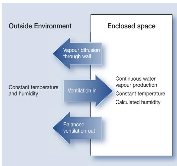
A simple algorithm was constructed in Excel examining moisture transfer by diffusion and ventilation. Basic relationships compatible with the CIBSE data for saturated vapour pressure and absolute humidity were employed.
