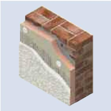
External wall insulation installed on a solid brick wall.
