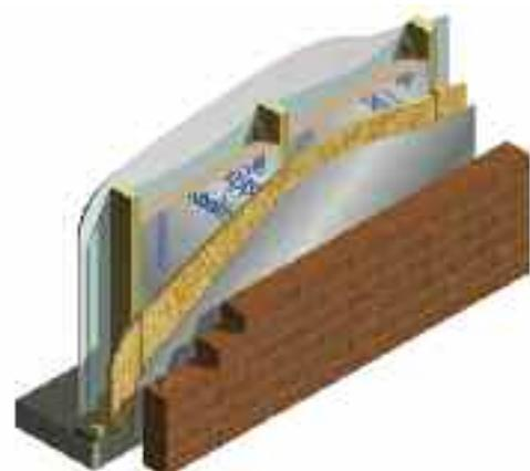
Wall 3 - Polythene Vapour Control Layer Added to Rigid Phenolic Insulated Wall
