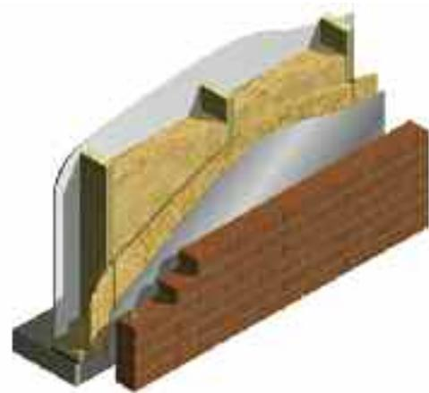
Wall 1 - Breathable Wall Insulated with 140 mm of Mineral Fibre Between 140 mm Deep Studs
